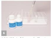
Add 1,000  $\mu$ L of the sample diluent to the red dilution cup and mix by pipetting up and down 5 times.
