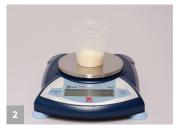
Obtain a representative sample. Grind and weigh out a 50 g sample.
