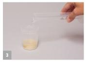
Add 250 mL distilled or deionized water to the sample.
