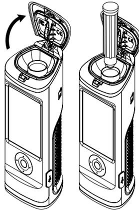
07. Close the door to depress the sampler and begin test. **Note:** keep instrument upright while the sample is being read.
