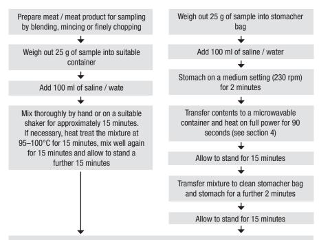
An amount of liquid should appear above a settled layer. Filter the liquid through a Whatman no. 4 or similar filter paper into a clean container. Alternatively a slurry may be obtained which may require centrifugation to obtain a suitable extract. Mix the sample extract, which is now ready for immunoassay.
