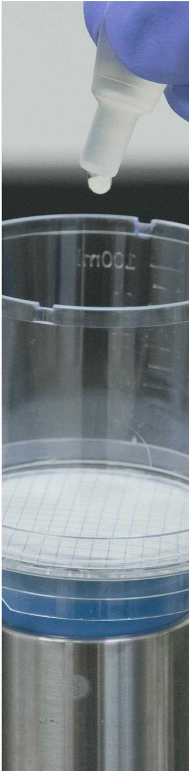
7. Remove and appropriately discard the plastic funnel. Place the filtration system cover over the filter/base assembly converting the unit to a petri dish for sample incubation.
