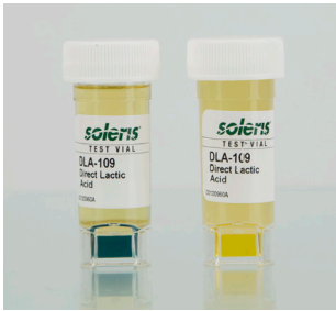
Soleris® vial uninoculated (left) and inoculated vial (right).
