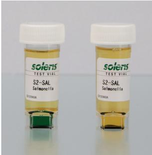
Soleris® vial uninoculated (left) and inoculated vial (right).
