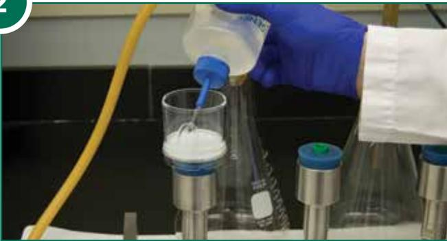
**Step 2 (optional):** Rinse the inside walls of the filter funnel with approximately 20 mL of sterile buffered solution. Apply vacuum just long enough to pull the solution through the filter, and turn off vacuum.
