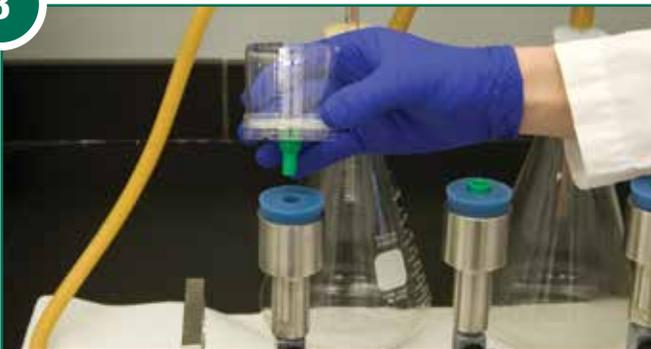
**Step 3:** Briefly remove the Neogen Filter and its funnel adapter from the rubber stopper to release any remaining vacuum pressure, and then re-secure into the stopper.
