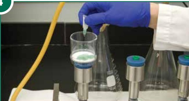
**Step 4:** Add the culture media onto the top of the filter. When doing so, be careful not to touch the filter with the tip of the ampoule.
