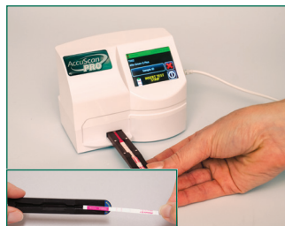
11. Remove promptly at 5 minutes and interpret results using the Reveal AccuScan Pro reader.
