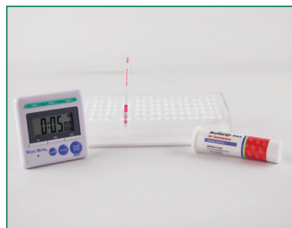
10. Place a new Reveal Q+MAX for Zearalenone strip into the sample cup. Set a timer for 5 minutes
