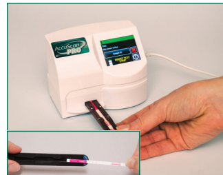
11. Remove promptly at 3 minutes and interpret results using the Reveal AccuScan Pro reader.
