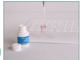
8. Add 1000 µL of sample diluent to the red dilution cup and mix up and down 5 times
