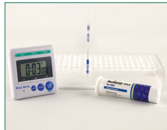
10. Place a new Reveal Q+MAX for DON strip into the sample cup. Set a timer for 3 minutes
